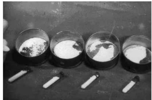
Picture 9 A marble chip from the Pietà compared to marble granules of various sizes.
