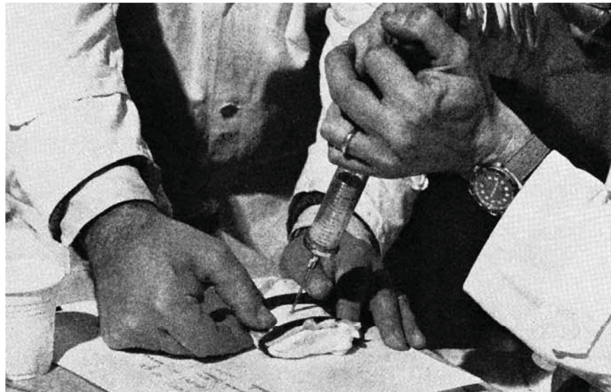
Picture 23 The compound of polyester resin and marble powder is injected between the cast and the mold in order to obtain, after resin catalization, the faux marble prosthesis.
